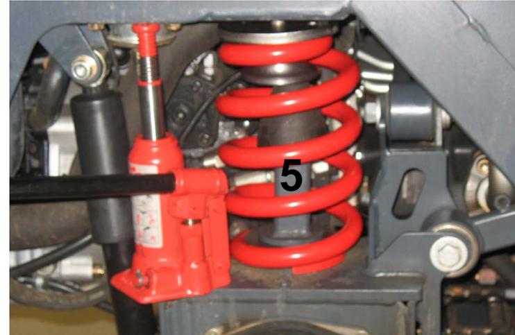
Note: There is no specified replacement interval for springs. The springs or the rubber buffer only need to be replaced when damaged. Always check their condition when carrying out maintenance tasks!
